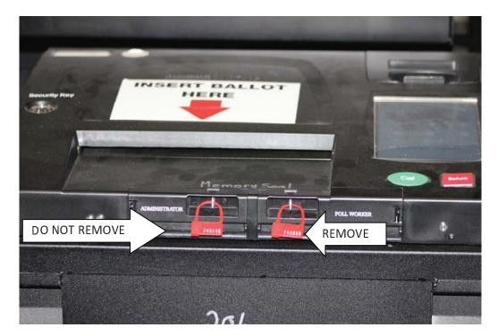
6. **Remove the memory card**: PUSH IN the small black button to the right of the card to release it, then, using a piece of tape (if needed) pull the card from the machine. AFTER YOU REMOVE THE CARD, MAKE SURE YOU SHUT THE DOOR SO IT DOESN'T GET BROKEN OFF WHEN THE FOAM IS REPLACED.
